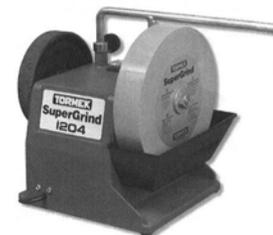
Many turners sharpen free hand, although a jig can help to keep consistent angles. A basic grinder with a grey wheel somewhere between 60 and 100 grit can achieve perfectly acceptable results with care.
