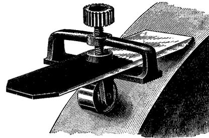
There are several honing guides on the market, varying in features. They all allow you to set and hold a consistent angle while grinding or honing the edge by hand on a flat abrasive surface. The angle of the blade to the flat surface is set by how much the blade projects beyond the front. They have a roller that contacts the abrasive surface to maintain the distance and corresponding angle of the blade to the surface.
