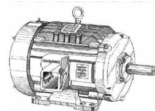
conduct heat away. TEFC motors are larger than open-frame motors for the same power output, but because they don't get clogged with sawdust, they need less maintenance. In the right conditions, a TEFC motor should last almost indefinitely.
