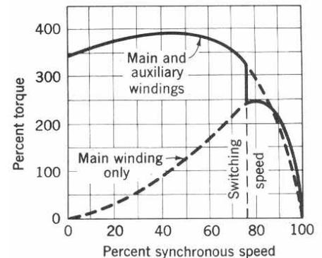
If the centrifugal switch fails, you may see starting problems or overheating of the motor, depending on whether it fails in the open or closed position.
