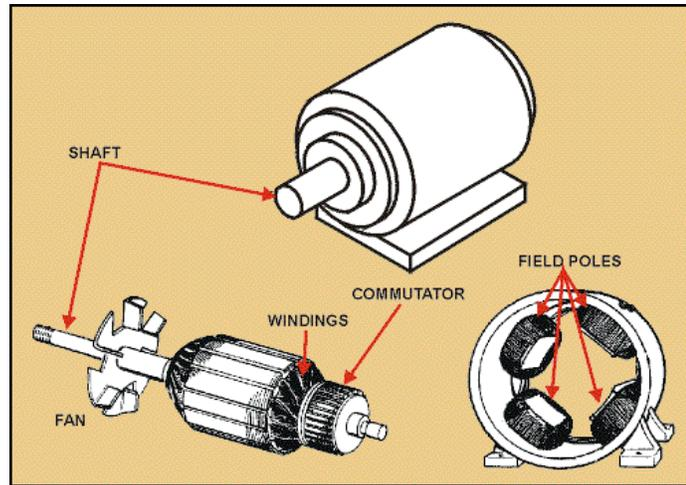
is the stationary field generated by the field poles, to provide the opposing magnetic field that generates the torque (turning force) that makes the rotor want to turn. In smaller motors, the field is created by permanent magnets such as on your battery screwdriver. In bigger motors, the field is an electro-magnet – it has copper windings as shown in the diagram. (See <http://www.claytonengineering.com/Training/myweb6/101basics.html> for more explanations.)
