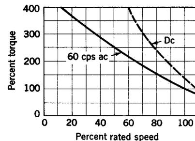
Fig. 11-12. Typical torque-speed characteristics of a universal series motor.
