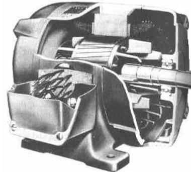
Open frame motors (see left) have holes for air to flow through for cooling – these are subject to clogging with sawdust like universal motors. Better motors for a dusty environment are the so-called TEFC (Totally Enclosed, Fan Cooled) motors (see right) that are sealed against dust and have a fan at the non-driving end that blows air over the motor to cool it. Some have fins on the outside, to help
