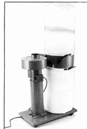
The one problem I encountered was the hang up of shavings on the inlet grid of the fan. For safety, the 100mm inlet to the fan has a coarse grid, to keep fingers and large objects out. However, shavings quickly become entangled with the grid, and then rapidly accumulate to block off the inlet pipe. This is particularly a problem when collecting shavings from my planer – the pipe can back up within a minute or two and has to be cleared out by hand.
