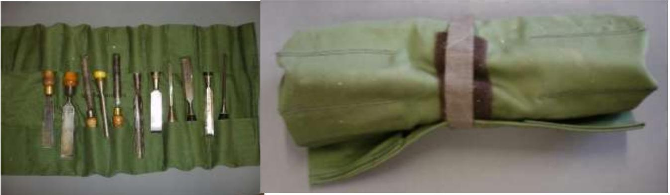
on the left, so then the roll is rolled from the right. The Velcro will hold it closed, for a variety of contents, giving different diameters. This one is 70cm wide by 35cm high. The 6cm pockets comfortably accommodate bench chisels. There are some smaller pockets on the sides of 3.5cm.
