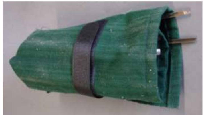
This is made from green canvas. Unfortunately, I didn't add a top flap to stop the tools from falling out the top. It is too short, with some longer tools inserted to show this. It is also a bit over-stuffed, and doesn't roll up nicely. Closure is with Velcro as above, which is quick and secure. It is 47cm wide by 18cm high, with 6cm wide pockets. This one needs reworking – I will make it taller and add a flap to fold down over the chisels.
