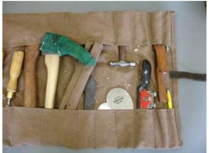
of tools in use. Due to the bulky tools included, it doesn't roll up nicely and looks rather awkward and over-stuffed. Brown denim is used, with a Velcro closure, which works well to accommodate the range of tools that could be fitted. Some extra pockets could be added for the flat scrapers. The draw-knife doesn't fit well into the pockets at present.
