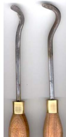
I tested the shapes with old screw-driver handles still attached, to decide whether it was worth proceeding. Once I was happy, I cut off the plastic handles and made a suitable wooden handles in a comfortable shape and size to suit, as you can see from the picture. Where the screwdriver shafts were moulded into the handles, two flanges could be seen, to locate them into the moulded plastic. I ground off the flanges. The handles were glued into the wooden handles using quickset epoxy glue.
