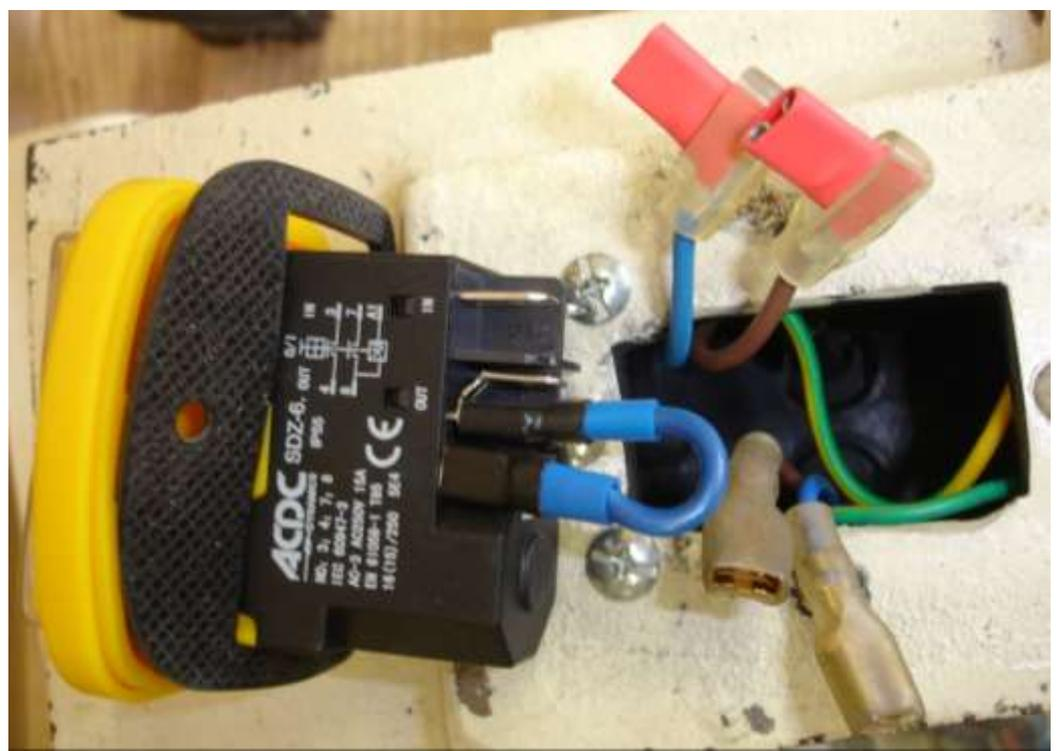
was simply reconnected using the same spade connectors as shown in the photograph. Red heatshrink was added to the incoming connectors to provide an extra degree of touch safety.
