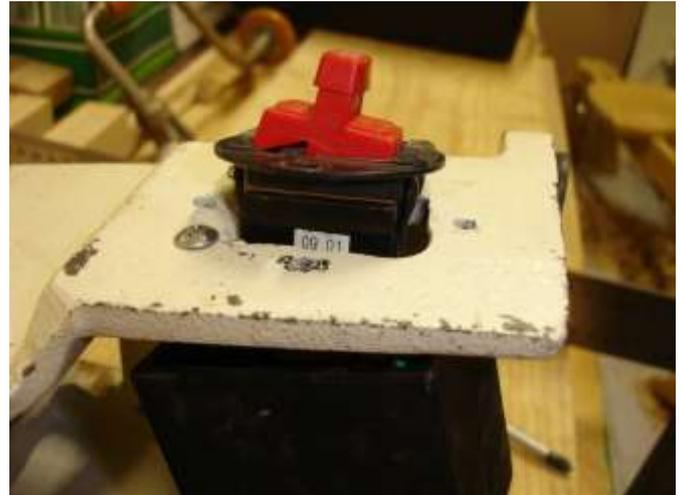
The OEM switch was a simple toggle switch, with a removeable key to prevent unauthorised use of the lathe if desired. The picture shows the switch partly removed. You can see the damage to the sides of the switch.
