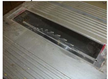
The downside of the throat plate is that it is not possible to fit the splitter and guard, as the throat plate would be too weak at the rear. Depending the type of cut I am making, I will either use the standard guard or fit the zero clearance throat plate.
