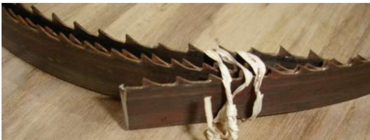
1. The teeth are very hard, which is a virtue, but it does mean that they can't be resharpened with a saw file as one might expect for hand saws.
