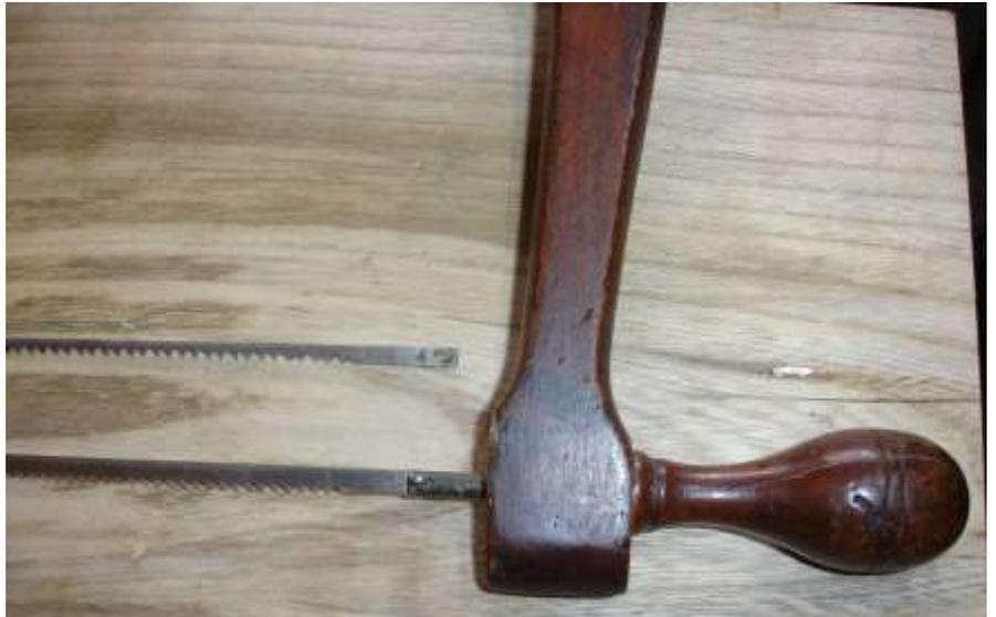
These old blades are resharpenable with a small triangular saw file. The blades were quite narrow to start with. With each sharpening, the blade will become narrower, as one would expect. You can see that the
