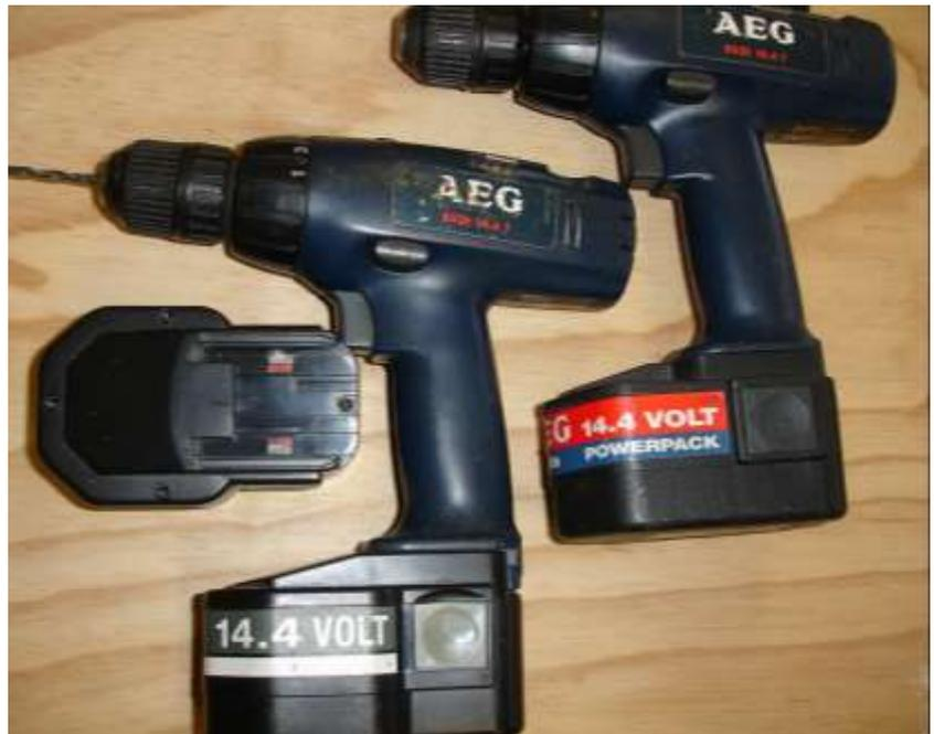
I managed to source two replacement packs from Battery Experts in 2015. These are 2.0 Ah packs, a higher capacity than the original 1.4 Ah pack. At the time, Battery Experts only had a branch in Durban, so they couriered them to me.
