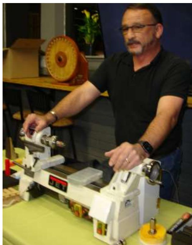
(You may be wondering what the lathe in front of Shane is. It is a somewhat modified Jet 1014, with the DC motor and variable speed electronics from a Nova Comet 2 added. There is also a spindle speed display above the switch buttons on the right. Mounted on the spindle is a collet chuck and mandrel for ring turning.)
