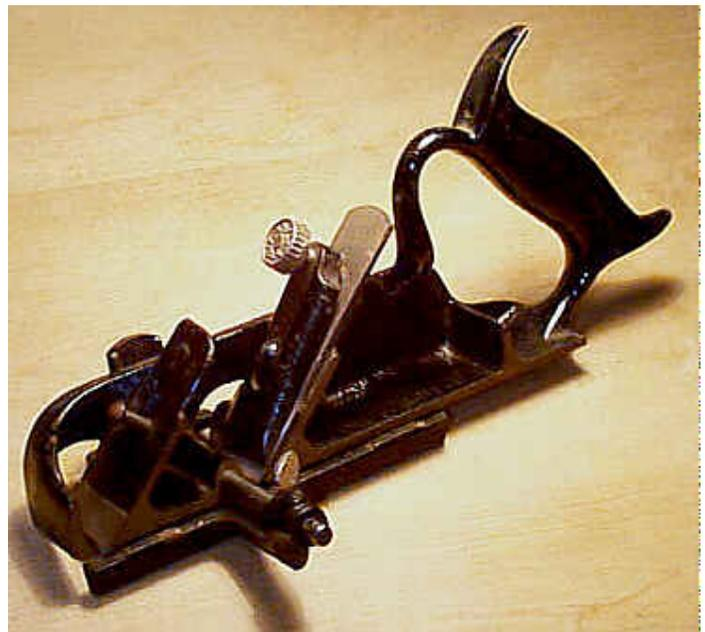
in 1925, a lever, which engages machined grooves in the backside of the iron, was provided to accomplish this. Around 1910, the handle has a fish scale-like pattern cast into it.
