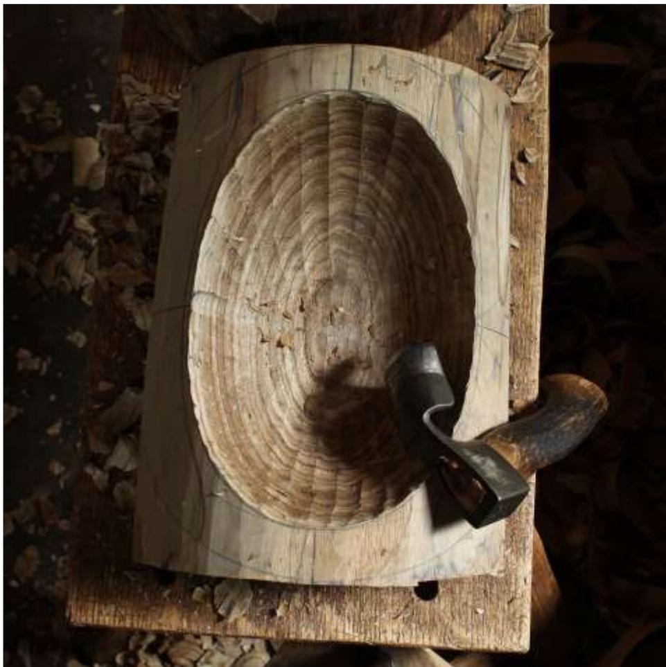
bevel on the edge should be on the inside or outside. The Pfeil that I have has the bevel on the inside and I am not sure about it. I haven't used it enough to form an opinion. The adzes that David Fisher uses for his hand carved bowls have the bevel on the outside, which makes them more useful for deep hollowing. This image
