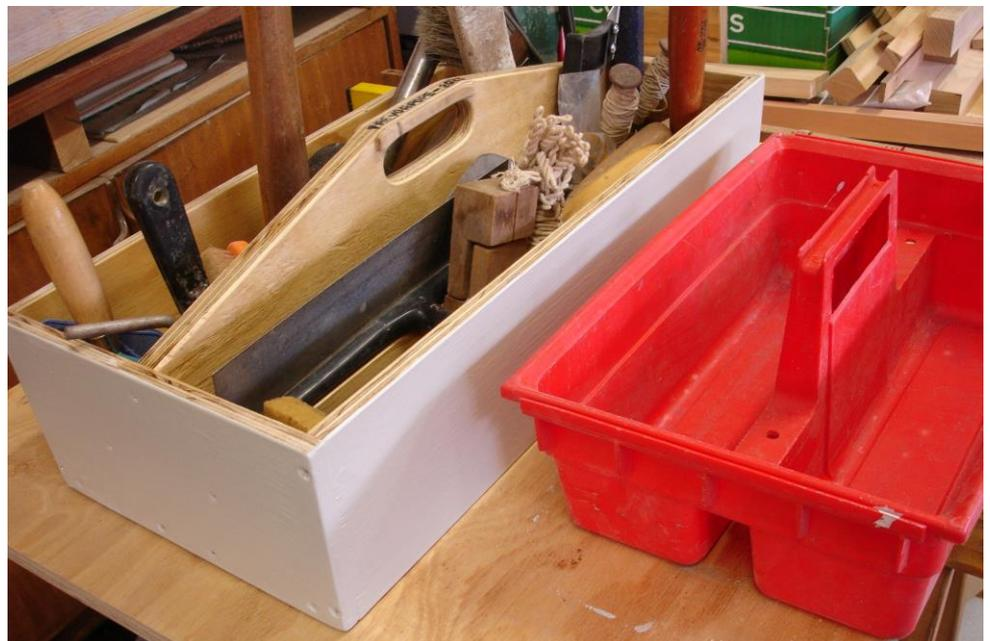
This is a top view of the new caddy. The interior dimensions are 52 cm long by 24 cm wide by 11 cm high. The height of the carry handle in the centre is 16 cm.
