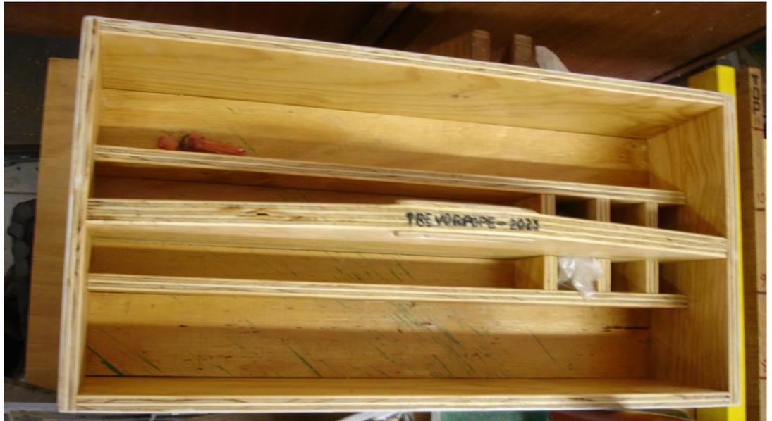
are placed close to the centre and some smaller dividers are placed at one end for small items and tools like chisels to stand up in. The centre divider and the two smaller dividers are let into shallow dados in the base to help with aligning them.
