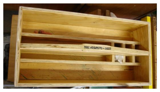
are placed close to the centre and some smaller dividers are placed at one end for small items and tools like chisels to stand up in. The centre divider and the two smaller dividers are let into shallow dados in the base to help with aligning them.
