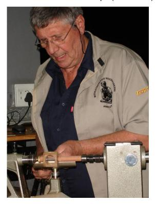
turned with 6mm tenons to match the 6mm hole drilled through the body. To make finishing the tenon end of the finials, Poena made a special live centre with a 6mm end and a pin for turning the tenons to size.
