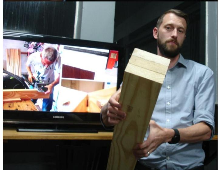
has a slab top of 1570l x 600w, laminated from pine. The legs, also laminated from pine are rebated into the top for a height of 900mm. 0.6m<sup>3</sup> of SA Pine weighing 280kg was used to make two benches. Dominoes were used to align the pieces for gluing.
