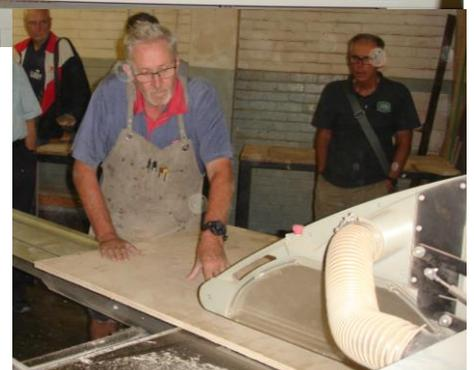
saw is square by making four successive cuts on successive sides of a piece of plywood.
