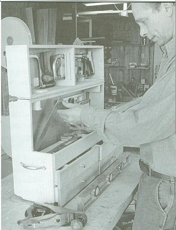
My design doesn't have drawers, but a deeper well that can accommodate a #7 plane and a 24" carpenter's square. The smaller Disston D-8 panel saws also fit in against the back wall.
