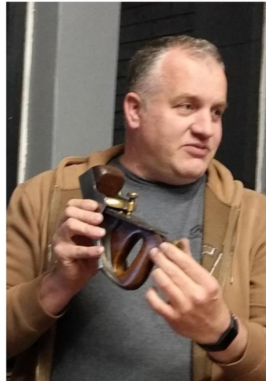
The photo on the right shows Mike holding a Norris infill smoothing plane – this design was mostly superseded by the Bailey pattern planes. The components of the Bailey pattern are shown in the diagram on the right.
